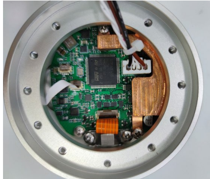
Figure 3-17 Wires that connect the wrist 3 joints to the end flanges
