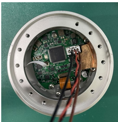
Figure 3-17 Wires that connect the wrist 3 joints to the end flanges
